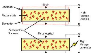
**Fig. 2:** Generation of piezoelectricity.
