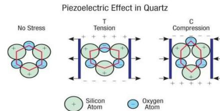
**Fig. 3:** Mechanism of piezoelectric effect in quartz
