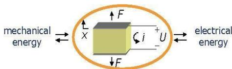
**Fig. 1:** Conversion of vibration/ mechanical energy into electrical energy and vice versa.
